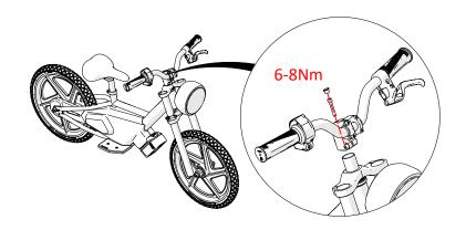
b. Align the stem with the front wheel and tighten the top cover screw with a locking force of 6-8N.m. After correct locking, please tighten the screws on two sides of the stem. Please refer to the value on the stem for the tightening force of the screws. Do not over-tighten the screws.
